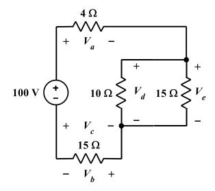
Use equivalent resistance and the voltage divider equation to determine each of the following:
